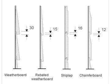
**Figure 1 Cladding Profiles**
