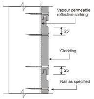
Figure 3 Shiplap or Chamferboard
